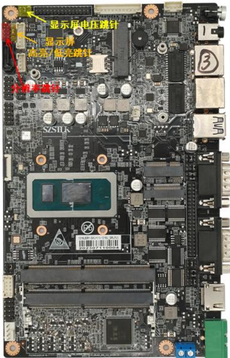
LVDS Display Brightness Jumper Settings(Chinese: 显示器高亮/低亮跳针):
